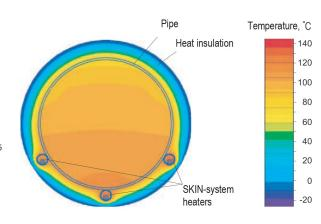
Example of heat insulated pipeline heating by three heating elements of SKIN-system with the total output of 130 W/m. Pipe diameter is 530 mm, tambient air.= -20°C
