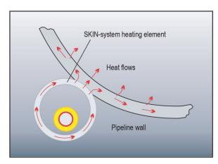
The conductor is electrically connected to the tube at the end of a heating run while AC voltage is sup-plied between the conductor and the pipe at the run head; the voltage value is calculated basing on the required heat output and the heated
