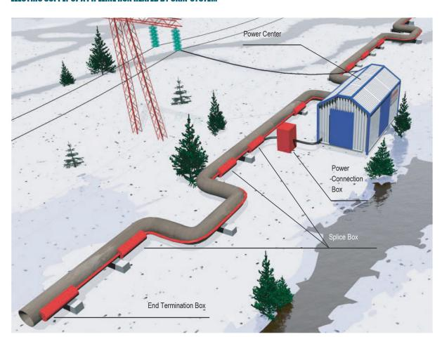
Electric power supply system is performed as an lancing transformer, monitoring and control system. uting sells of the HV and LV sides, specialized ba- tically sealed and heated container.
